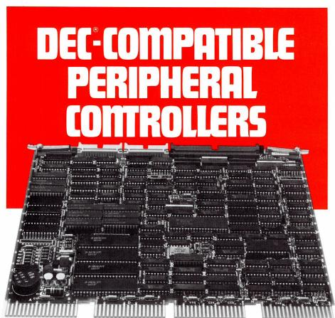
LSI-11<sup>®</sup> compatible controller for 80-300MB CDC, Ampex and Fujitsu CMD/SMD
