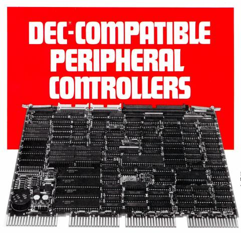
LSI-11® compatible controller for 80-300MB CDC, Ampex and Fujitsu CMD/SMD
